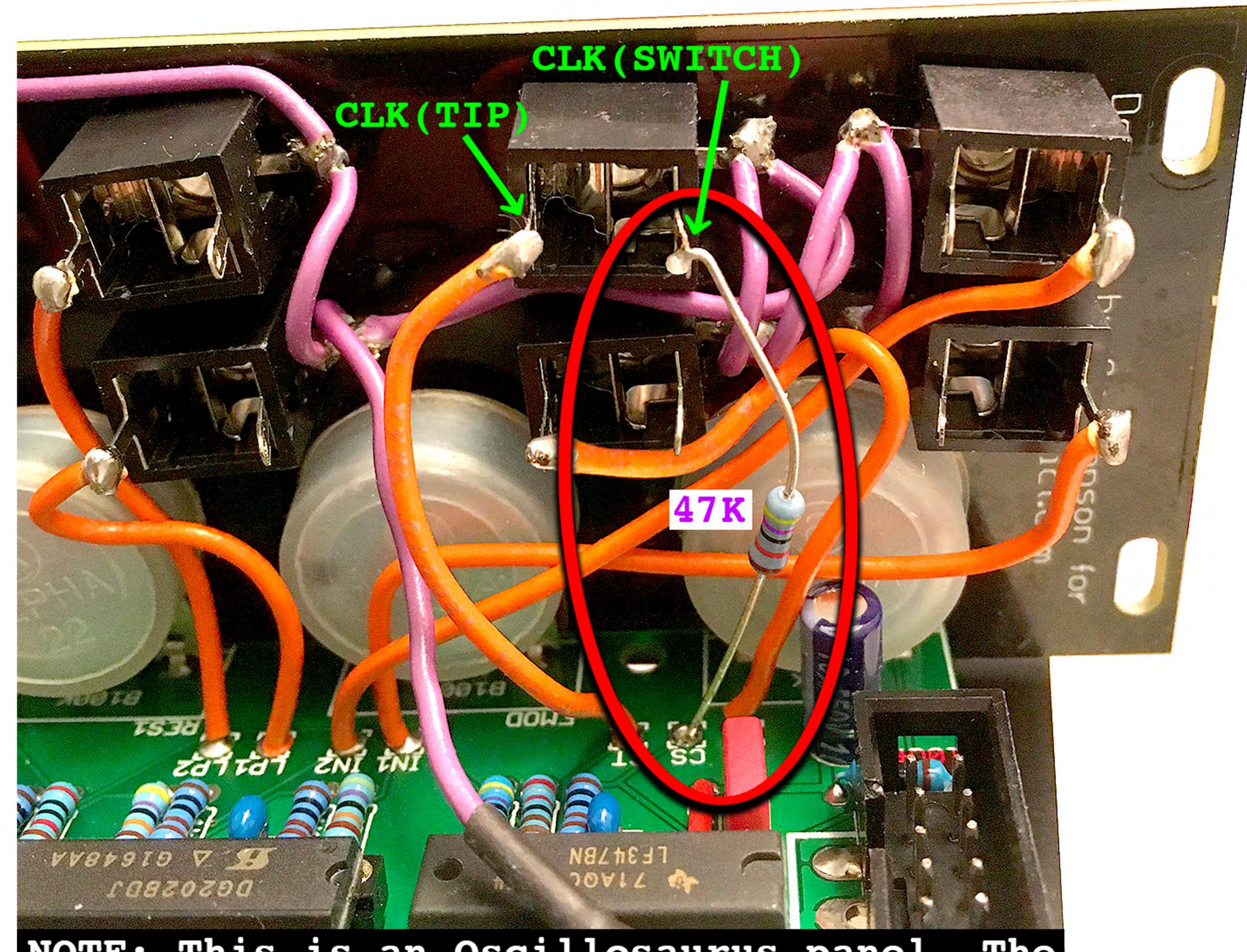
NOTE: This is an Oscillosaurus panel. The location of the jacks are different from what is shown in the Barton Build Docs
