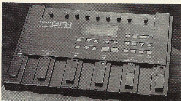
Roland's GR-1 uses voltage, rather than MIDI, to trigger its onboard sounds from the GK-2 pickup, evading tracking delay problems. Its MIDI Out also lets it control external synths and signal processors.
