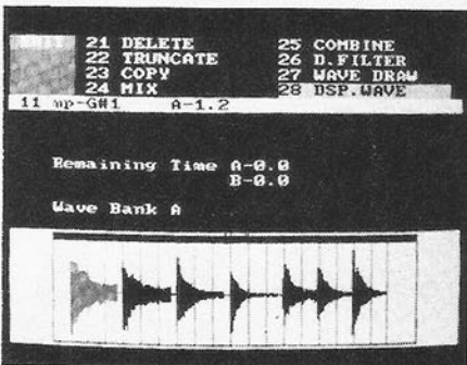
Display of samples in bank A. The currently selected sample is highlighted in color (grayed out here). Remaining sample time is shown at center screen.
