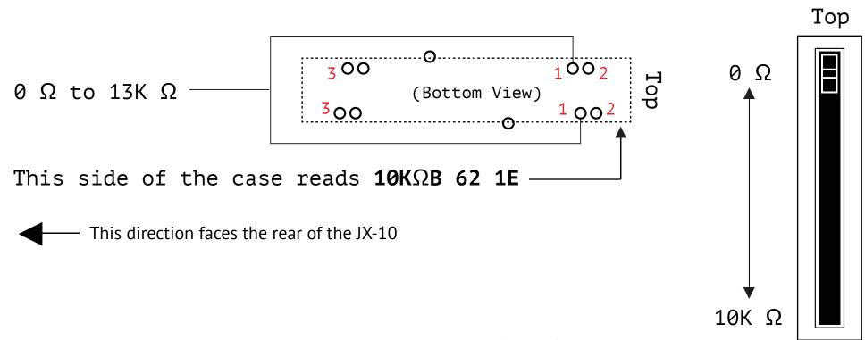
It was not unusual to find a higher value of 13K  $\Omega$  when it was measured. This could be due to age, dirt or manufacturing tolerances
