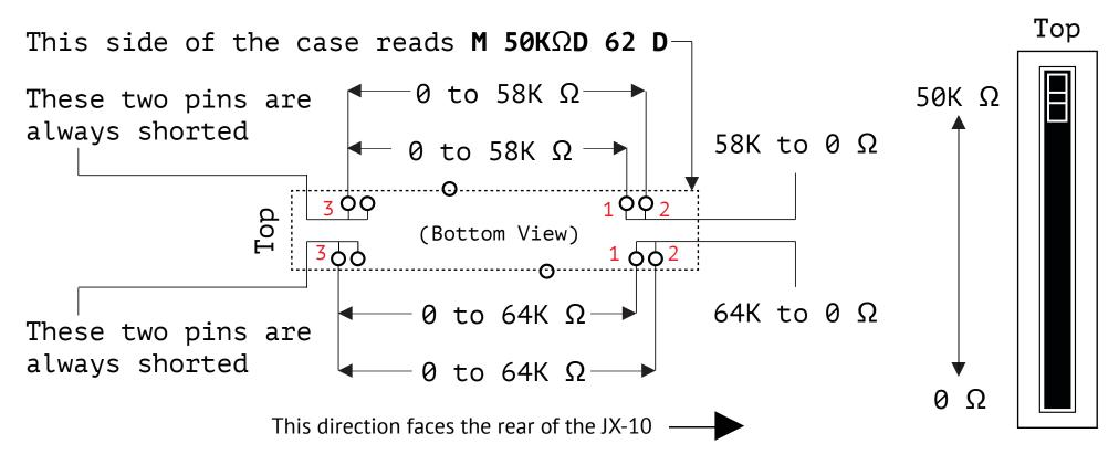
It was not unusual to find higher values of 58K  $\Omega$  and 64K  $\Omega$  when it was measured. This could be due to age, dirt or manufacturing tolerances
